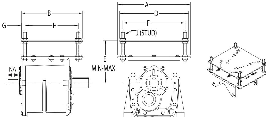
The MAXUM XTR Motor Mount is a rugged fabricated steel assembly which requires no drilling or foundation. It bolts directly to the reducer and accommodates a wide variety of NEMA AC motor frames.
