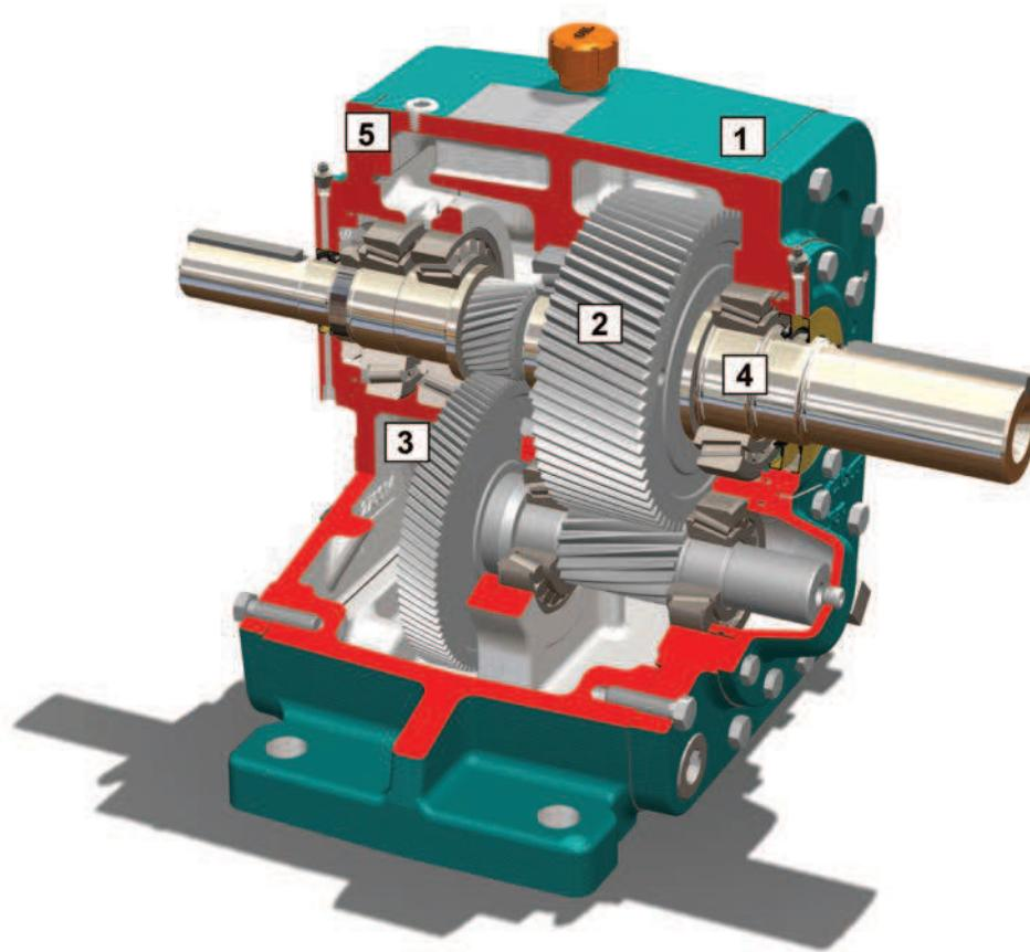
1. **Housing** - Rugged ductile iron, compact design with increased stiffness to provide dependable performance in less space. Condition monitoring pads are standard for the mounting of accelerometers.
