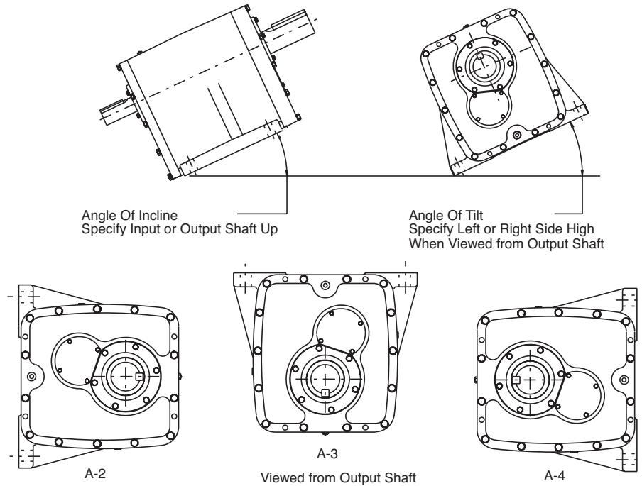
DODGE MAXUM XTR Concentric Shaft Reducers can be modified to permit mounting in positions other than the conventional (A-1) floor mounting. Some of these include ceiling (A-3) and wall (A-2 and A-4) and various inclined, vertical and tilted positions. Consult factory to determine what modifications are required for your specific application.
